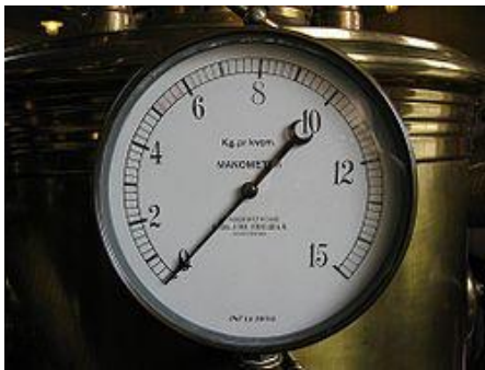
Figure 3 (left) Bourdon gauge (right) Mechanism of the Bourdon gauge
